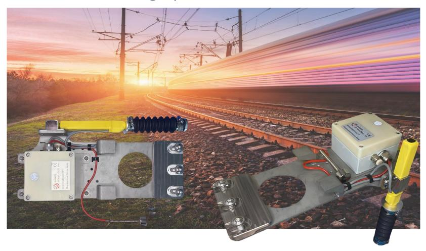
This internally powered dual sensor node allows remote measurement of dynamic distance displacement associated to track voiding and critical rail temperature (CRT) monitoring utilising a magnetic probe which measures the rail skin temperature.
