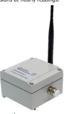
WiSenMeshNET nodes communicate via bespoke encrypted mesh radio technology can be up to 400m from each other or the SmartGateway. The sensors mesh together and automatically form a network relaying data off each other (up to 10 sub mesh levels of data hop) and back to a central data hub called a SmartGateway which contains the data logging functions, radio mesh control systems and external communication to the WiSen cloud-based datacentre or local hosted system.
