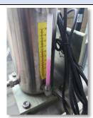
Figure. Liquid Level Settlement Node.
