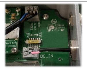
Figure. 110-240VAC to 12VDC@5A Adapter Connection.
