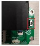
It can be switched on/off before/after a node's power-on. This pointing mode only becomes active after a valid laser reading is achieved.
