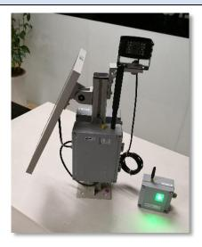
Figure. Camera Node (Left) & Visual Node (Right)
