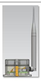
Figure. Mini Gateway Product Photo and the relate USB Connection.
