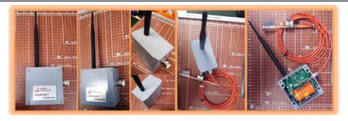
Figure. 1-Channel VW Interface Node Product Photos.
