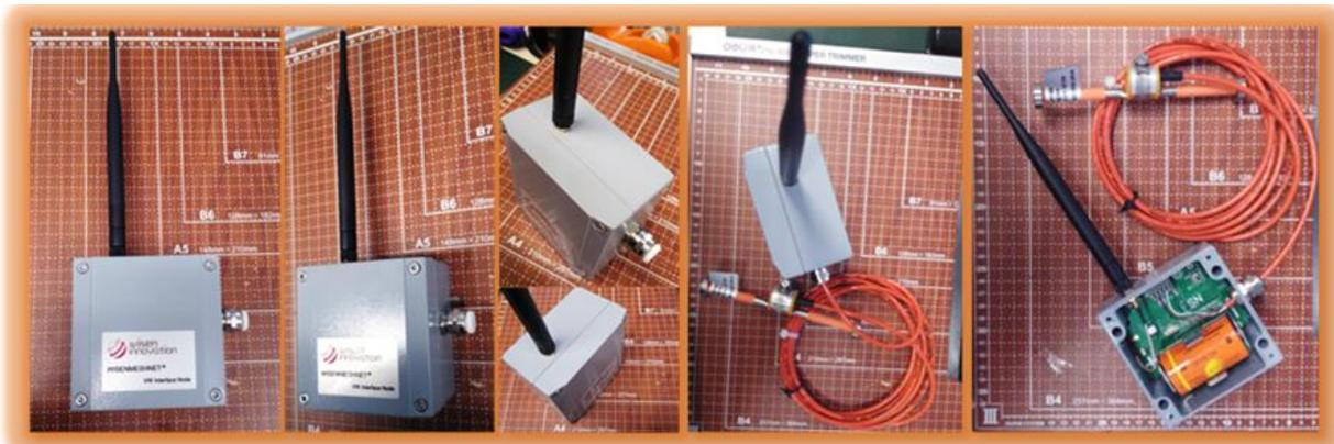
Figure. 1-Channel VW Interface Node Product Photos.
