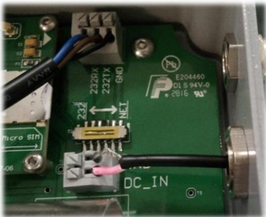
Figure. 110-240VAC to 12VDC@5A Adapter Connection.
