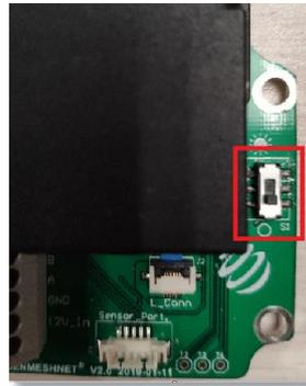
It can be switched on/off before/after a node's power-on. This pointing mode only becomes active after a valid laser reading is achieved.
