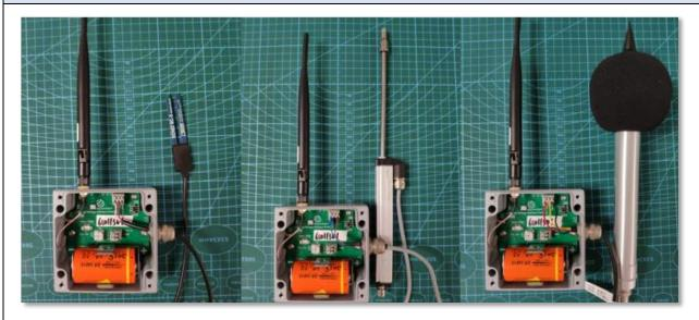
Figure. Voltage Node (From left to right: EC-5 Soil Moisture in %, Displacement in mm, Noise Level in dB).
