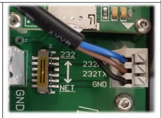
Figure. RS232 to USB Connection.
