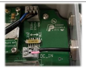
Figure. 110-240VAC to 12VDC@5A Adapter Connection.
